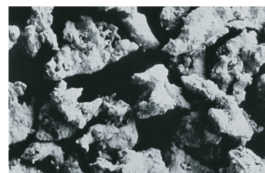
Ametek P316L Stainless Steel Filter Powder screened to precise mesh sizes for optimum spinning quality and throughput.
