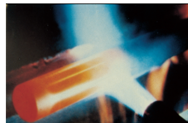
Powders sizes for all torch configurations make spraying hardfacing powders easier.
