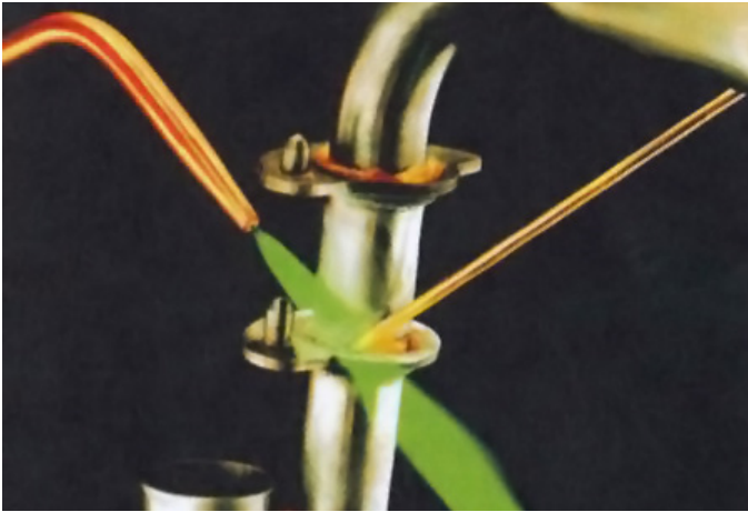
Yellow Stop-Off for Torch Brazing image source: AWS Brazing Handbook P. 238
