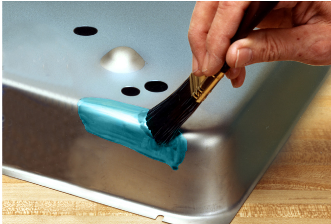
Blue Stop-Off brushed onto surface part
