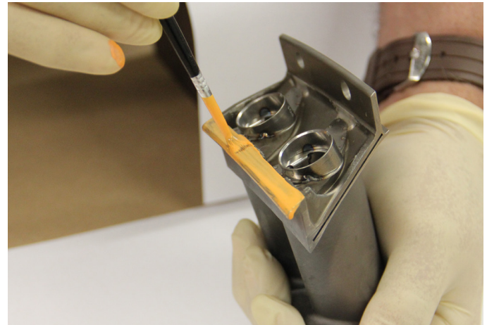
Orange Stop-Off brushed on vane segment
